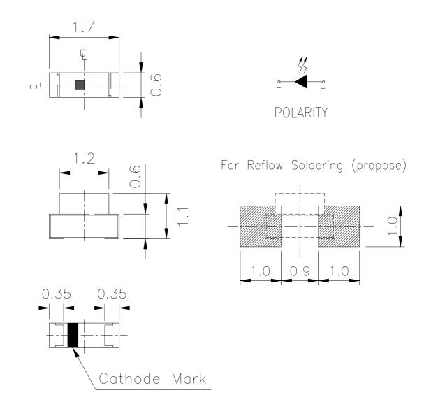
Note: The tolerance unless mentioned is  $\pm 0.1$  mm, unit is mm.
