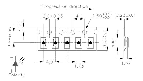
**Note:** The tolerance unless mentioned is  $\pm 0.1$  mm, unit is mm.
