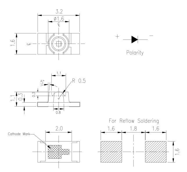
**Note:** The tolerance unless mentioned is  $\pm 0.1$  mm , unit is mm.
