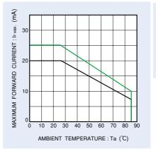
SML-521MYW<Green> SML-521MDW<Green> SML-521MUW<Green> SML-521MVW<Yellow> SML-521MDW<Orange> SML-521MUW<Red>
