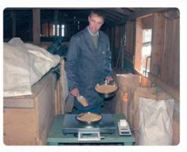
Thanks to the formula function various components of a mixture can be weighed together. In order to check, the total weight of all components can be called
